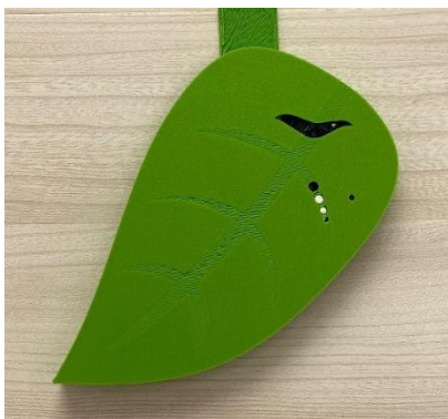
Fig. 2. SmartMe next-gen sensor for the indoor monitoring of air parameters.
